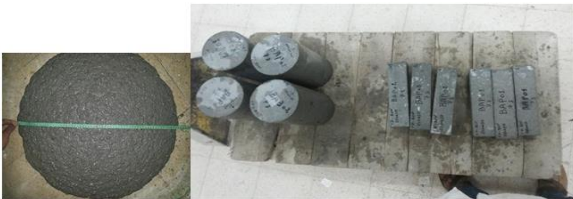
Figure 3: Slump test and samples of concrete
