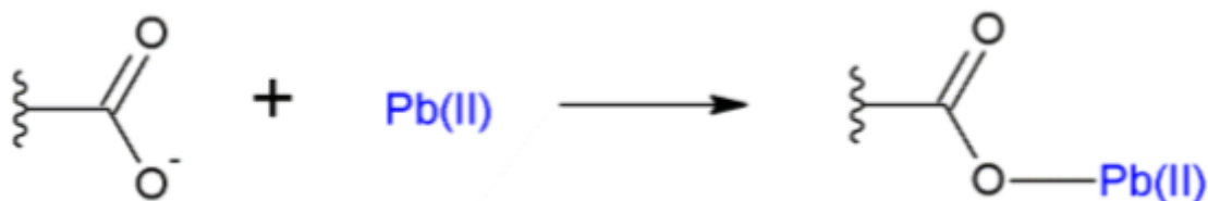
Figure 1: Monodentate coordination of Pb(II) ion with the carboxylate group in CPHB
