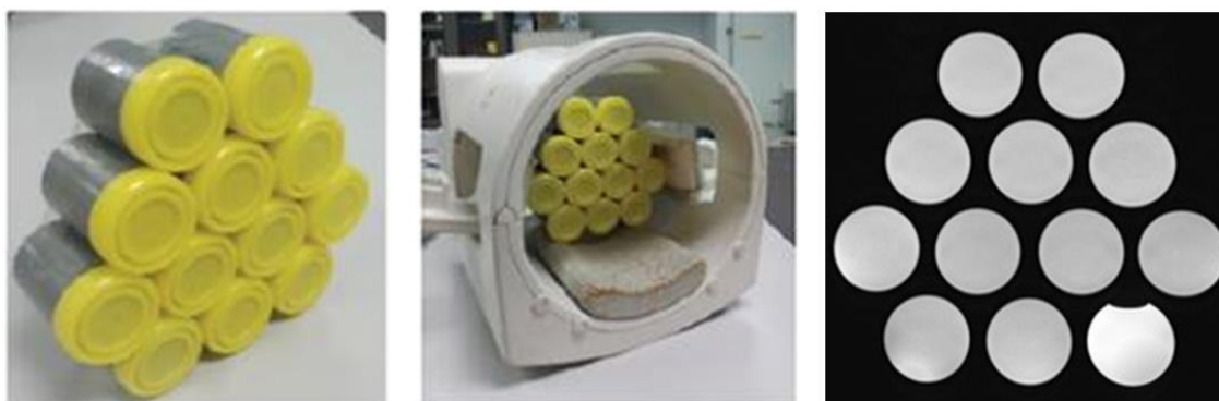
Figure 1: MRI phantoms (Left) when positioned horizontally inside the RF head-coil (Middle) and the images obtained (Right)
