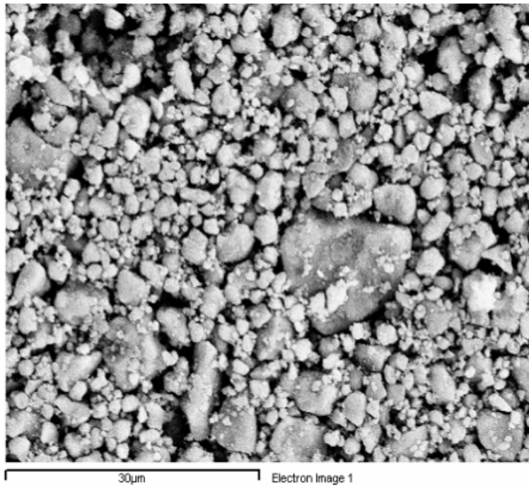
Figure 2: SEM micrograph of carbonated apatite precursor powder
