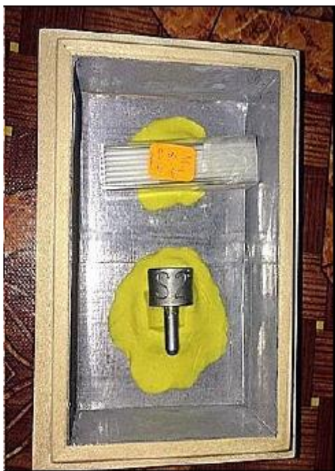
Figure 9: Shows the shield box that contains milk sample and the radioactive source
