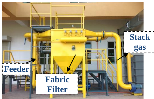
Figure 1: a) Pilot plant fabric filtration system.
