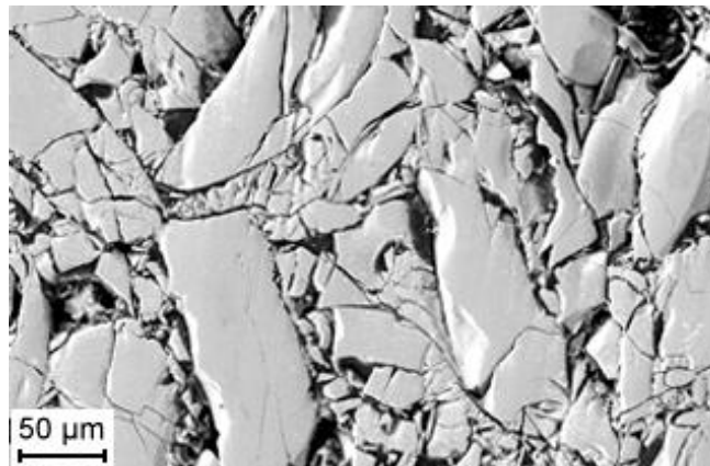
Figure 3(a): Electron micrograph of compacted bonded magnet. Magnification 200x.
