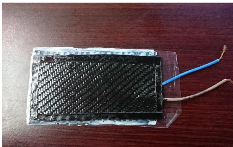
Figure 2: A sample of developed organic photo-supercapacitor with 20gsm paper soaked in \text{Na}_2\text{SO}_4 [sample of size (10cmx4.5cm), mass 0.009kg]
