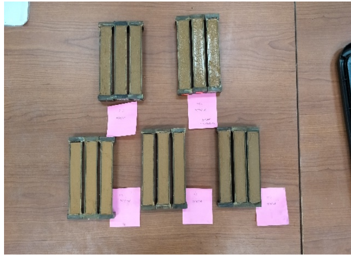
Figure 6. The Shrinkage test of soil-geopolymer mixture
