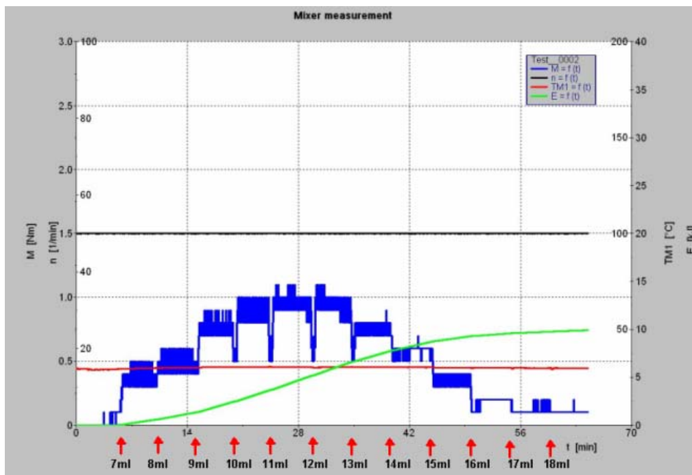
Figure 1: The torque curve for determination of powder loading
