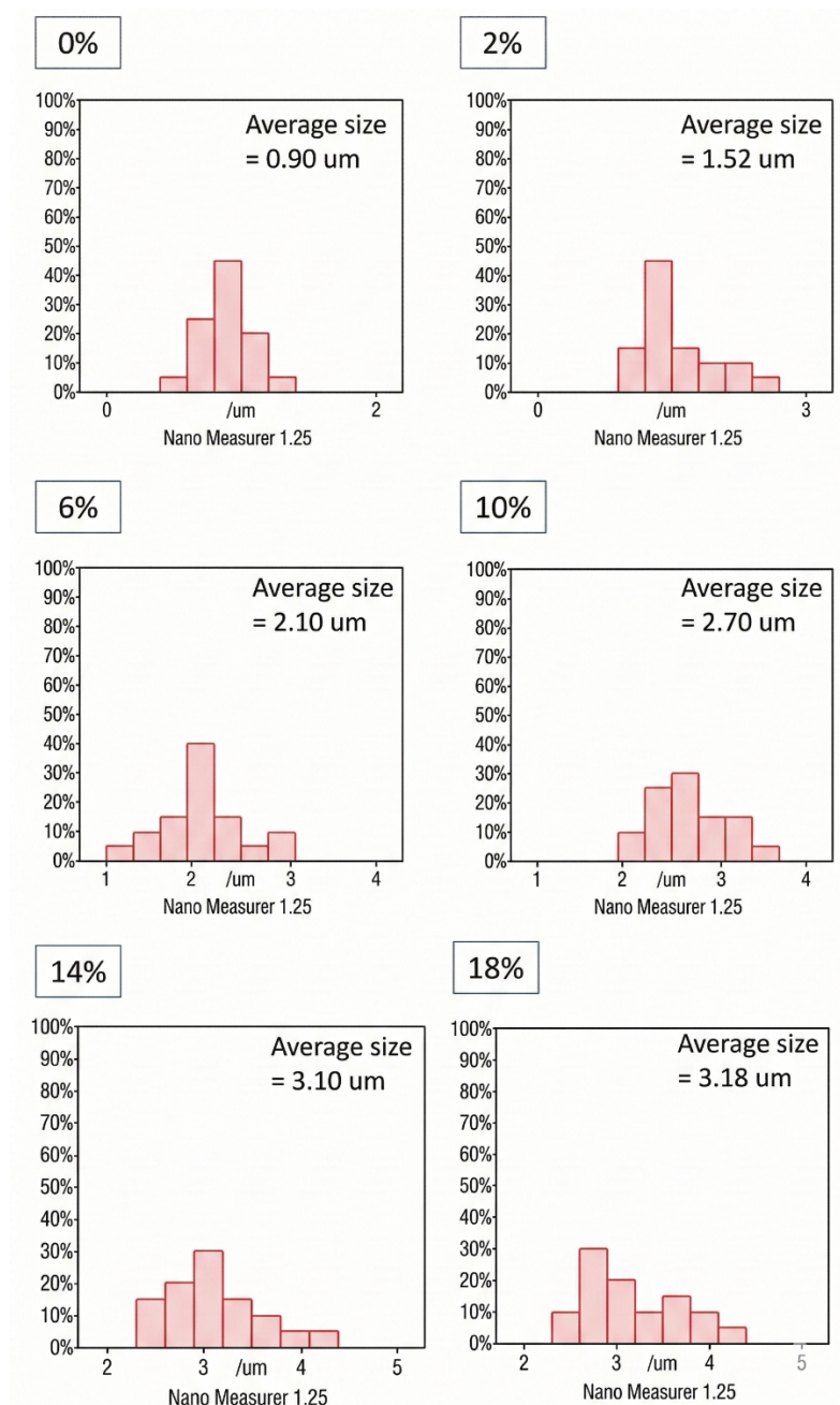
Figure 5. Particle size distribution in the form of histograms for undoped and Dy (2, 6, 10, 14 and 18 mol%)-doped ZnO nanocrystals
