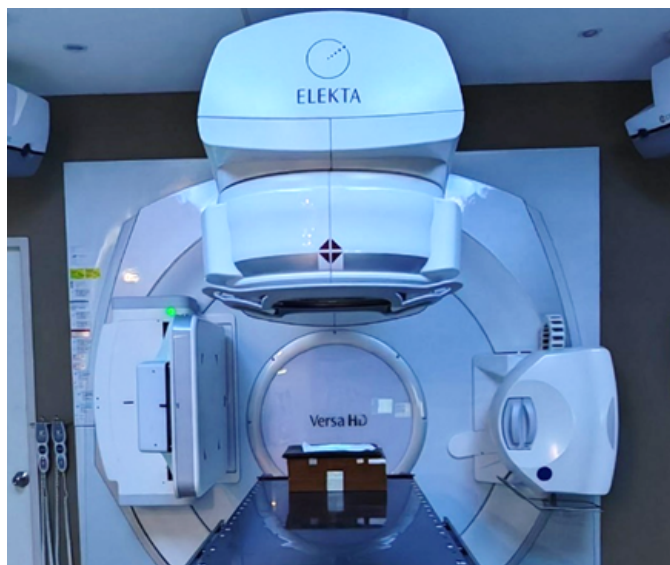
Figure 2. The irradiation setup showing the arrangement of TLD-100 chips, solid water phantom slabs, bolus material and 6 MV photon beam from the linear accelerator
